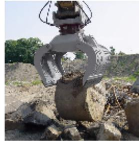
The DD02H is a 2000 and 2000kg capacity grapple for the Brokk 90 and 180.
