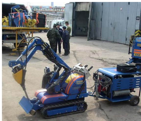
Brokk 40 with breaker and generator set
