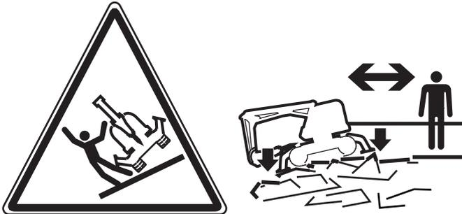
*Risk of compression or crushing injury. Outriggers must be deployed when working. Anchor the machine. Keep your distance*
