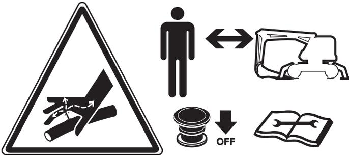
*Risk of personal injury. Keep your distance. Rest the arm system against the ground. Switch off the motor. Read the manual*
