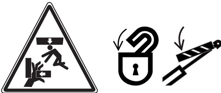
*Always mechanically secure moving components before disconnecting screwed joints or hydraulic hoses*
